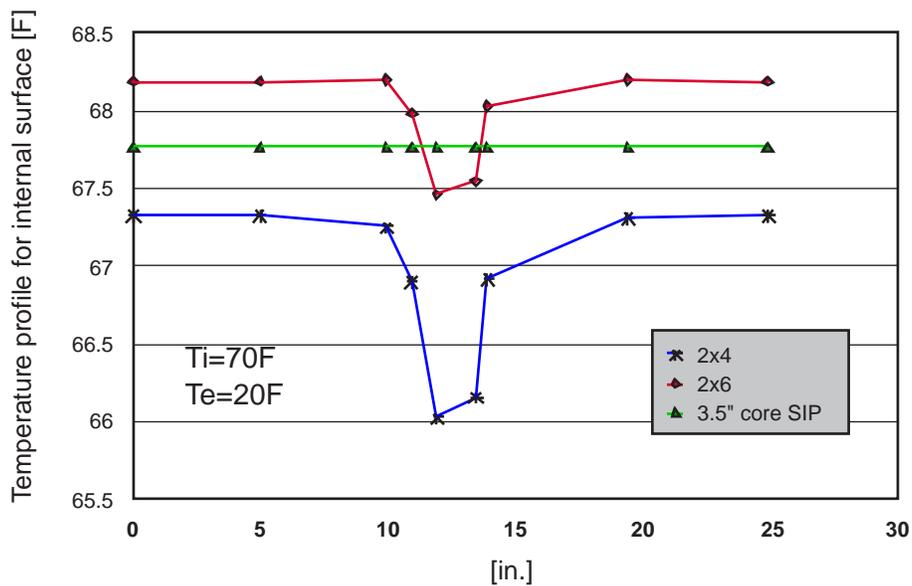
Figure 4. Local temperature comparisons for SIP wall and conventional 2x4 and 2x6 wood frame walls.
