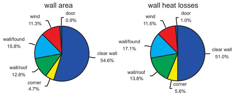
Figure 8. Wall area and wall heat losses distributions for SIP wall system with "best practice" details.
