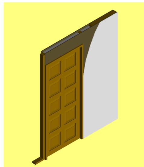
Figure B6. SIPA wall system—door header R-value =  $13.59 \text{ h} \cdot \text{ft}^2 \cdot \text{°F/Btu}$ , range 1.0 ft; door jamb R-value =  $13.59 \text{ h} \cdot \text{ft}^2 \cdot \text{°F/Btu}$ , range 1.0 ft.
