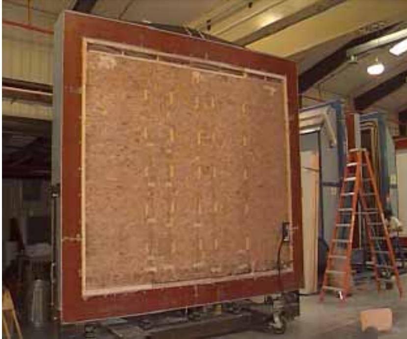
Figure 1. SIP wall prepared for hot box testing.
