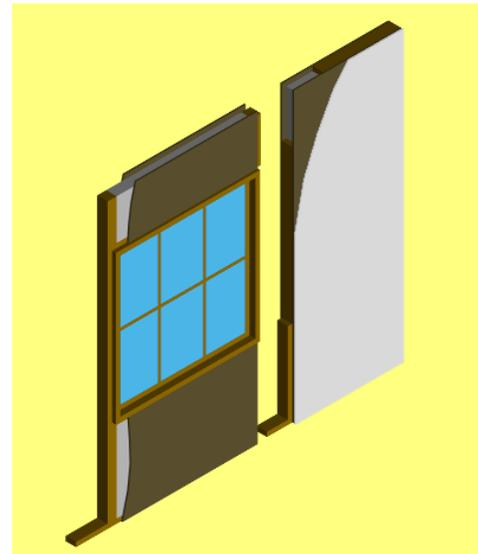
Figure B5. SIPA wall system—window header R-value =  $13.23 \text{ h} \cdot \text{ft}^2 \cdot \text{°F/Btu}$ , range 1.0 ft; window jamb R-value =  $13.23 \text{ h} \cdot \text{ft}^2 \cdot \text{°F/Btu}$ , range 1.0 ft; window sill R-value =  $13.23 \text{ h} \cdot \text{ft}^2 \cdot \text{°F/Btu}$ , range 1.0 ft.
