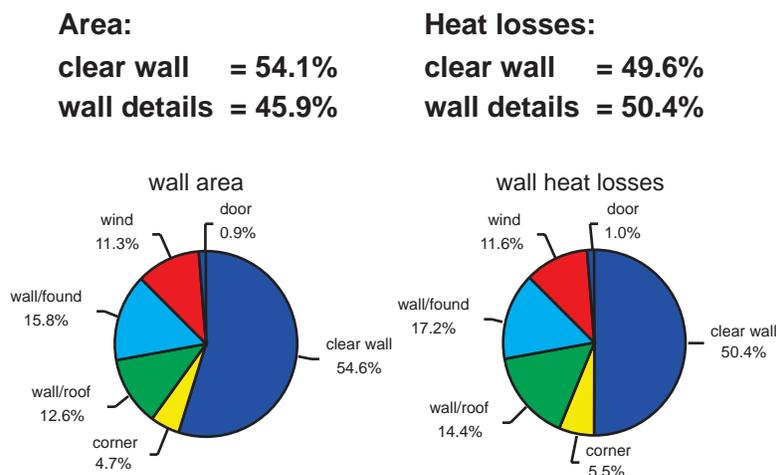
Figure 7. Wall area and wall heat losses distributions for SIP wall system.
