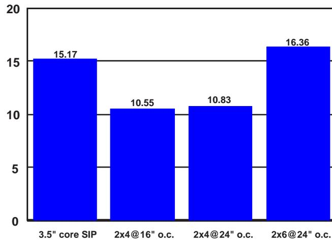
Figure 3. R-value comparisons between SIP wall and conventional 2x4 and 2x6 wood frame walls.
