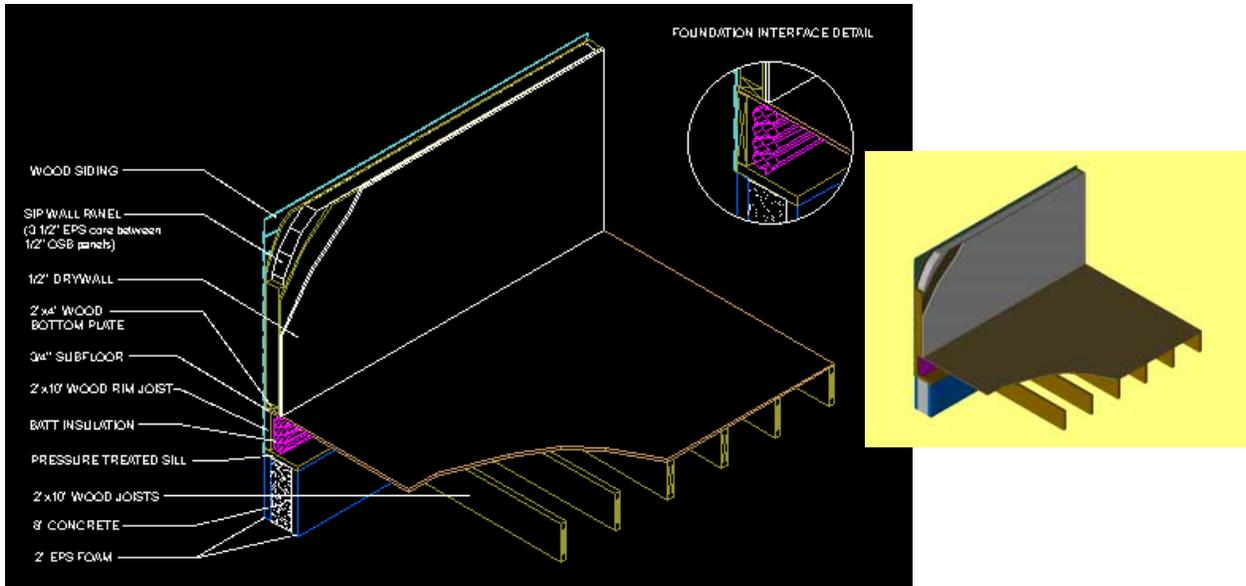
Figure B4a. SIPA wall system—foundation/wall intersection—typical detail (R-value =  $12.92 \text{ h} \cdot \text{ft}^2 \cdot \text{°F/Btu}$ , range 1.08 ft).
