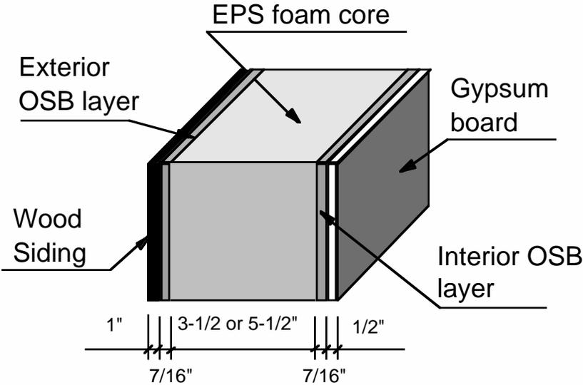
Figure 2. SIP wall section with finish layers.
