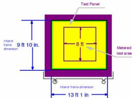
Figure A2. ORNL Buildings Technology Center hot box test panel schematic.
