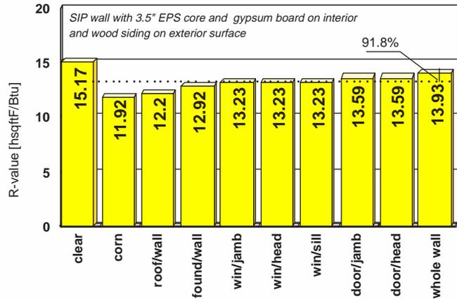
Figure 5. Whole wall R-values for SIP wall system with 3.5" EPS core.
