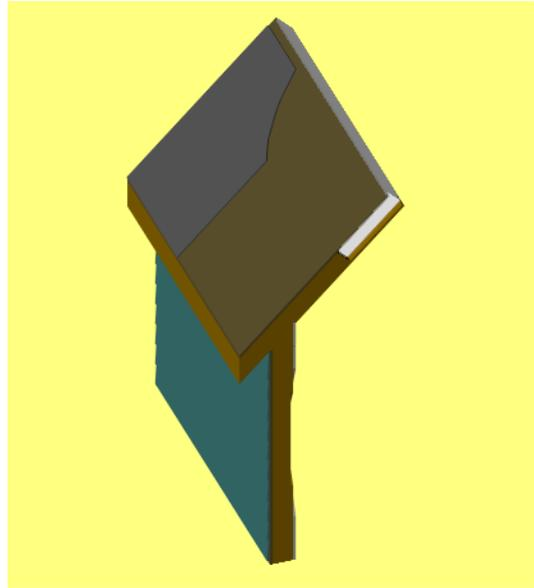
Figure B3a. SIPA wall system—roof/wall intersection—typical detail
