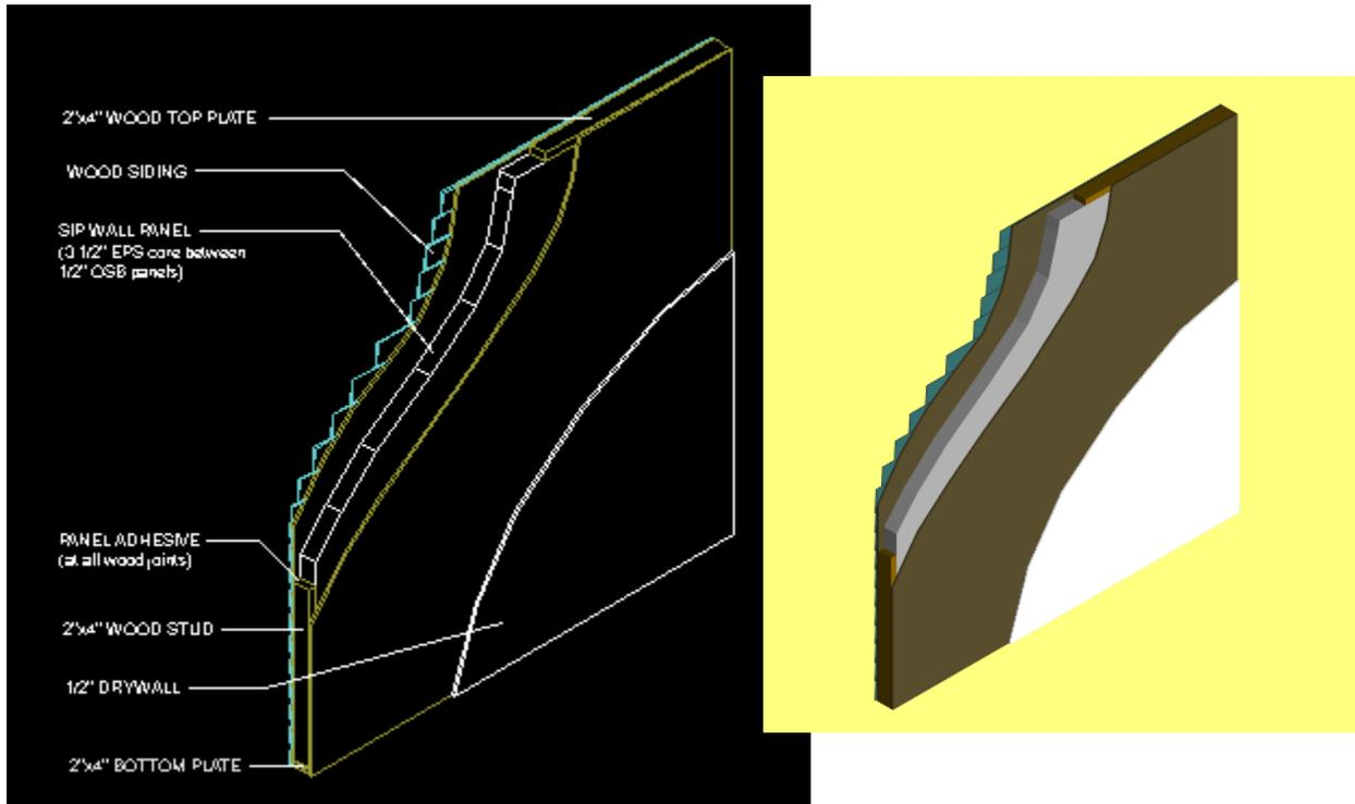
Figure B1. SIPA wall system—clear wall area ( $R\text{-value} = 15.17 \text{ h} \cdot \text{ft}^2 \cdot \text{°F/Btu}$ ).
