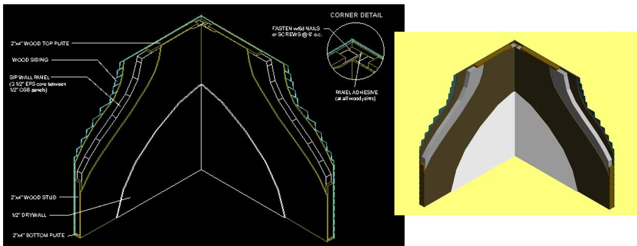
Figure B2. SIPA wall system—corner ( $R\text{-value} = 11.92 \text{ h} \cdot \text{ft}^2 \cdot \text{°F/Btu}$ , range 1.67 ft).
