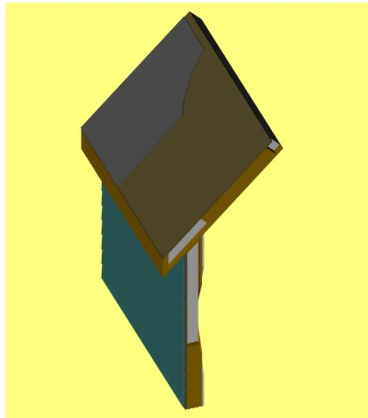
Figure B3b. SIPA wall system—roof/wall intersection—best practice detail
