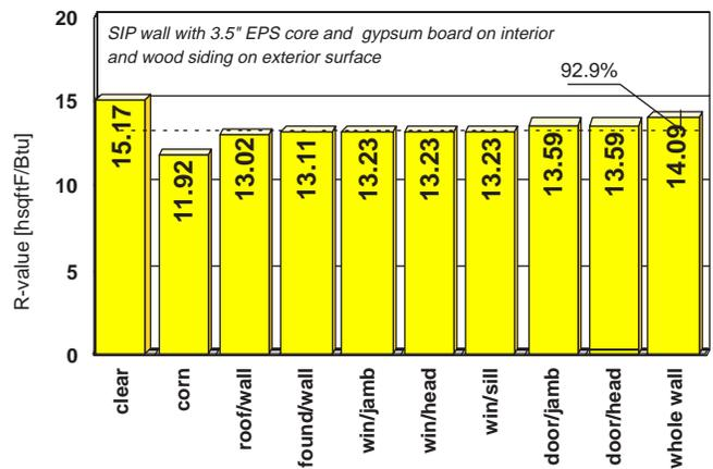
Figure 6. Whole wall R-values for SIP wall system with 3.5" EPS core and the "best practice" details.
