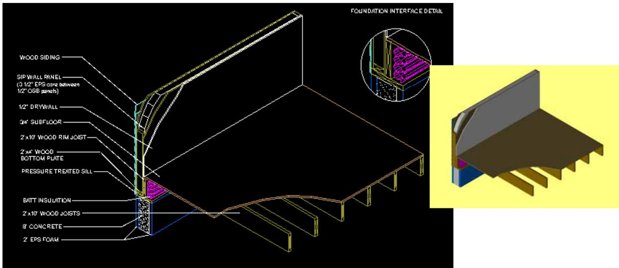
Figure B4b. SIPA wall system—foundation/wall intersection—best practice detail (R-value =  $13.11 \text{ h} \cdot \text{ft}^2 \cdot \text{°F/Btu}$ , range 1.08 ft)
