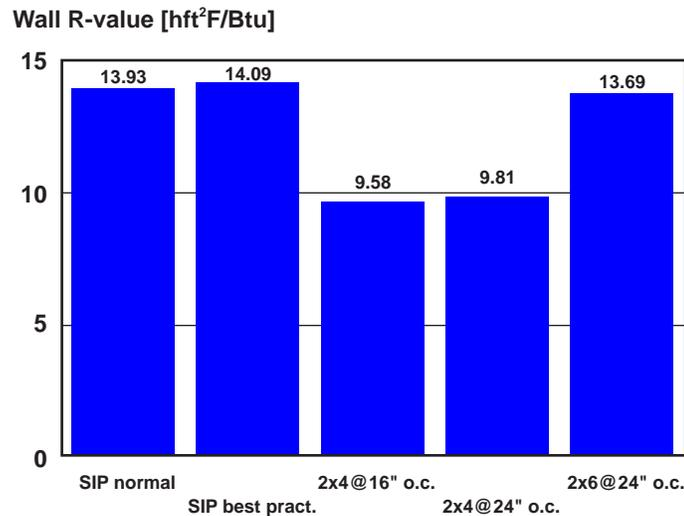
Figure 9. Whole wall R-value comparisons between 3.5" core SIP wall and conventional 2x4 and 2x6 wood frame walls.
